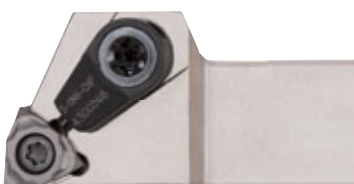
External coolant supply (at normal pressure)
