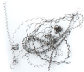
External coolant supply (at normal pressure)
